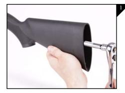
Begin by removing the existing recoil pad from your stock using a phillps head screwdriver. Next using a long flat head screwdriver or the appropriate socket with extension remove the stock bolt from the inside of the opening in the rear of the stock as seen in Figure 1.
