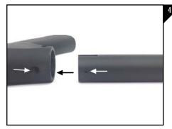
Next, insert the adapter tube into the rear of the pistol grip and align the pre-drilled hole on the top of the grip with the one in the tube as seen in Figure
