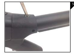
Using the provided 8-32 x 1/2 Flat Head Torx Screw and a T20 torx driver (not provided), tighten the buffer tube to the pistol grip as seen in Figure 5.
