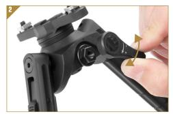
Pull the lever out and rotate the exposed hex nut clockwise to increase and counterclockwise to decrease the amount of tension applied by the lever.
