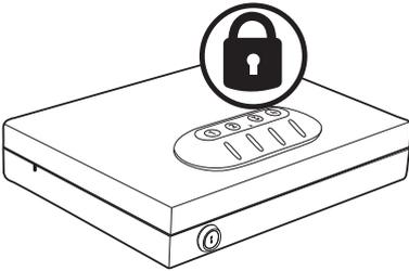
1. Three consecutive incorrect code entries will put the vault in “Basic Lockout” mode. Touch pad is deactivated for 30 seconds.
