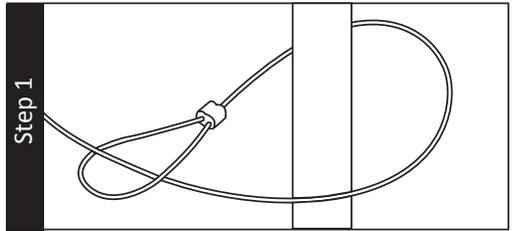
2. Place the cable's free loop into the notch on the side of the vault while still opened. Locking the vault with the cable loop inside will secure the cable inside the vault. Check the loop to ensure there is no way it can be manipulated to be easily removed from the fixed object, before leaving unattended.
